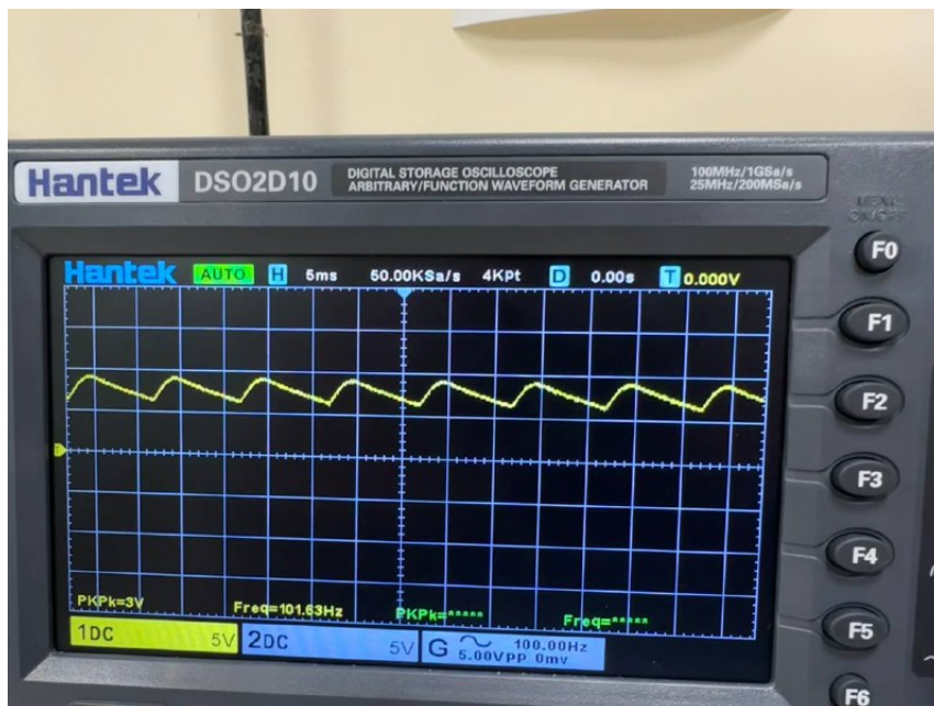
Figure 6: Normal diode rectifier with 2.2\mu F capacitor
